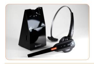
Wireless Base Station Unit. The base station connects via the handset port of the user's telephone and aligns the pin configuration with a simple switch. It sends and receives RF signals to a paired wireless headset. When a headset docks with the unit, it immediately pairs with it and also charge it.
